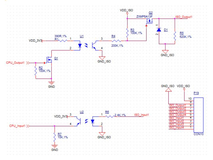
Isolated GPIO reduced schematic
