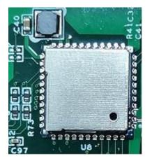
Figure 390: RTL8821CS WiFi/BT Module
