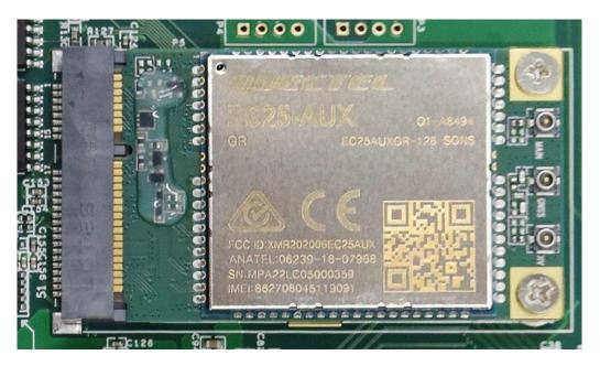
mini-PCIe Connector & 4G/LTE Module
