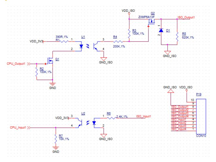
Isolated GPIO reduced schematic
