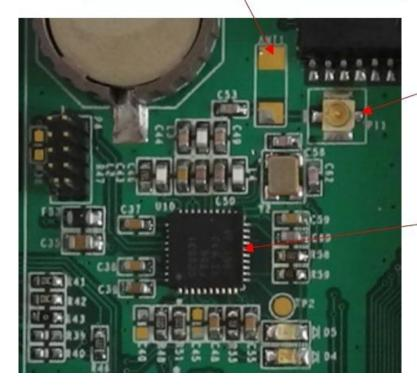
External Zigbee Antenna Connector
