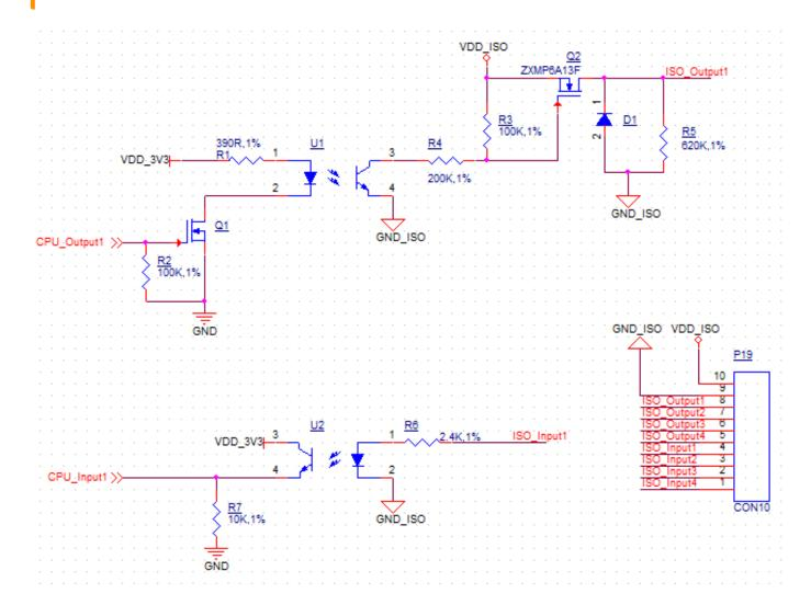
Isolated GPIO reduced schematic
