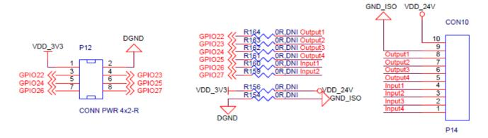
CPU GPIO Reduced Schematic
