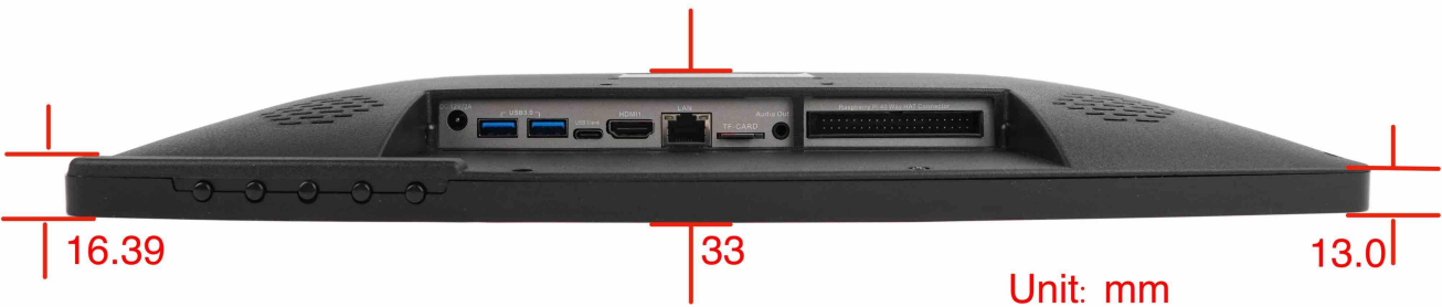
Side Dimension Technical Drawing
